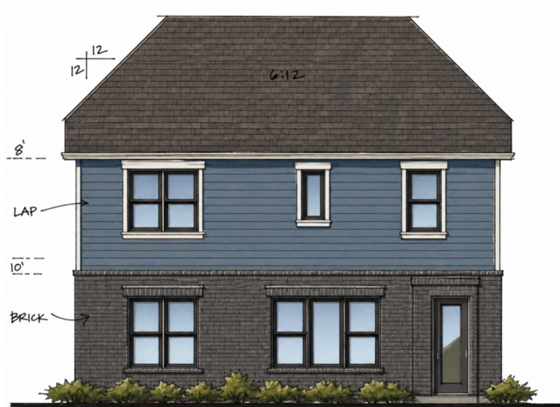
REAR ELEVATION OF 45' WIDE LOT (TRANSITIONAL STYLE)
